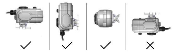
Flow can go in both directions. The position chosen for the installation should allow for accessibility to the valve during operation, inspection and maintenance.
