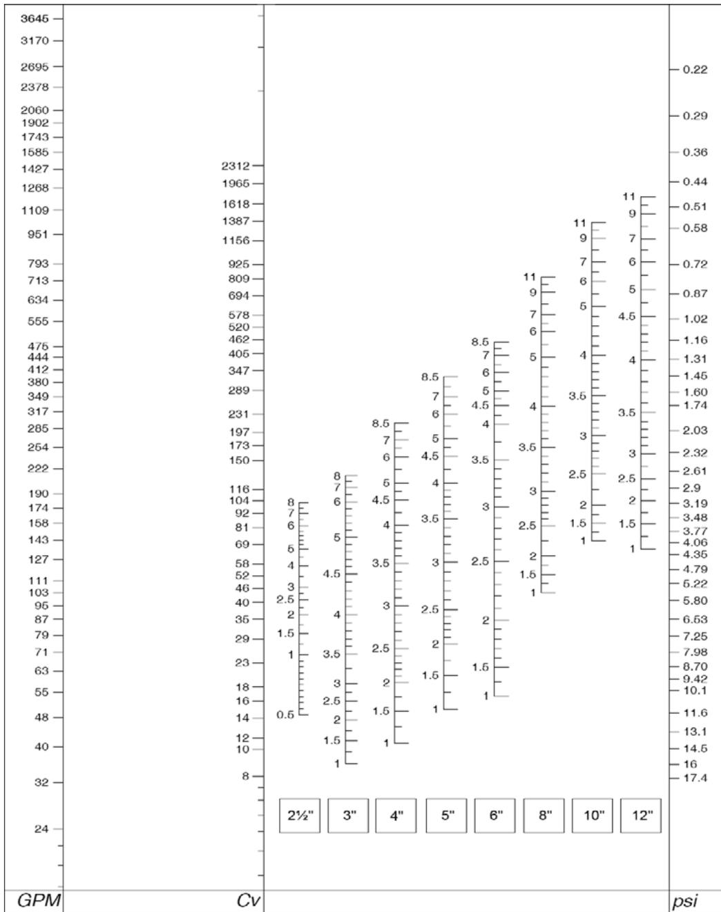
Using the diagram above, it is possible to determine the presetting position of the valve with the given design flowrate and headloss:
