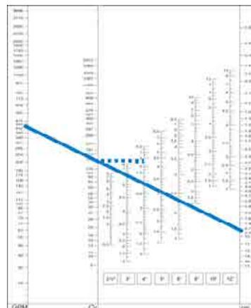
In the example for a design flowrate of 440GPM and design  $\Delta p$  9.4psi handwheel position of 5.6 is determined for a 4" valve
