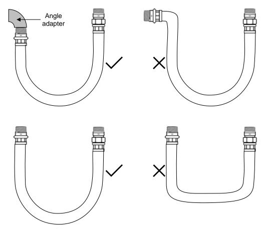
To prevent damage to the connections, torque during assembly must not exceed hand-tight plus a quarter turn. NOTE: Over-tightening of the threaded connection on the swivel end may cause cuts in the compression gasket, resulting in leakage past the compression gasket.
