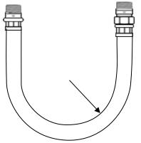
Whenever the bend radius falls below the indicated values, an angle adapter should be used to remove the sharp bend. In addition always keep the hose radius as large as possible.
