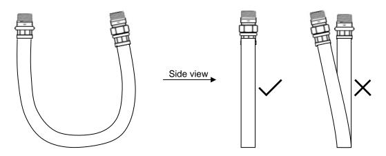
Sharp bends must be avoided. Hoses should NOT be bended to a radius lower than that indicated in the following table. If coil hoses are stored or installed at temperatures of  $40^{\circ}F/4^{\circ}C$  or lower, the bend radius should be increased by 50%.
